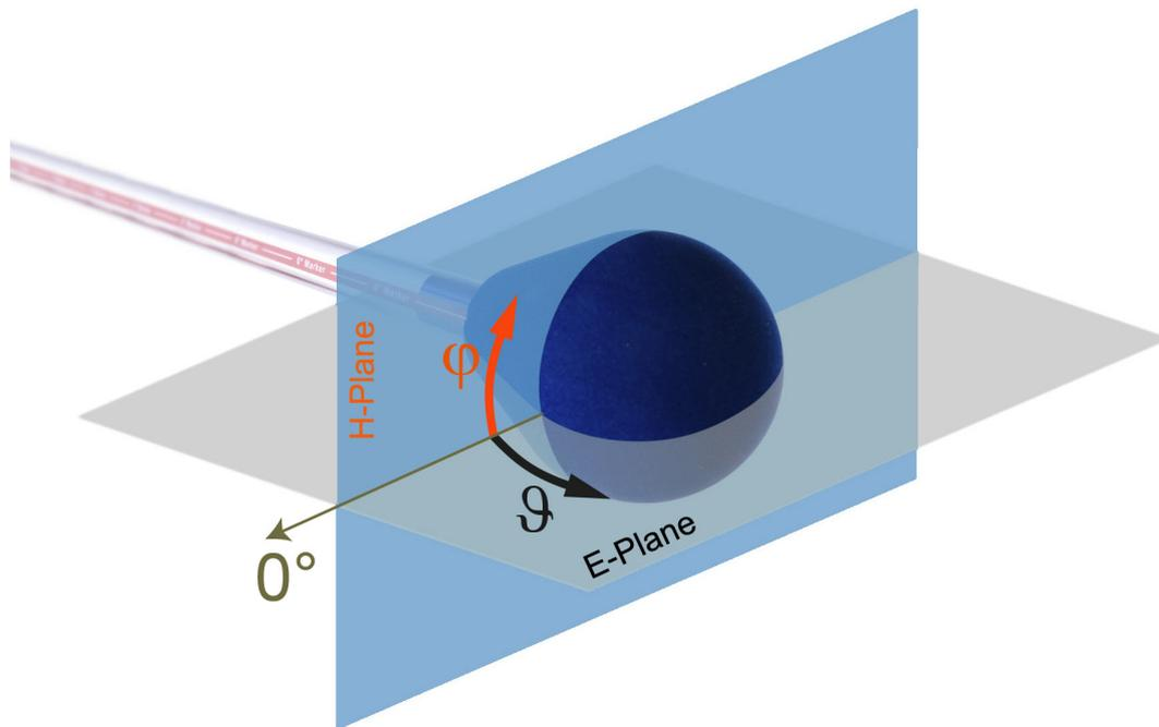
**Figure 15:** Definition of E- and H-planes for the radiation pattern diagrams
