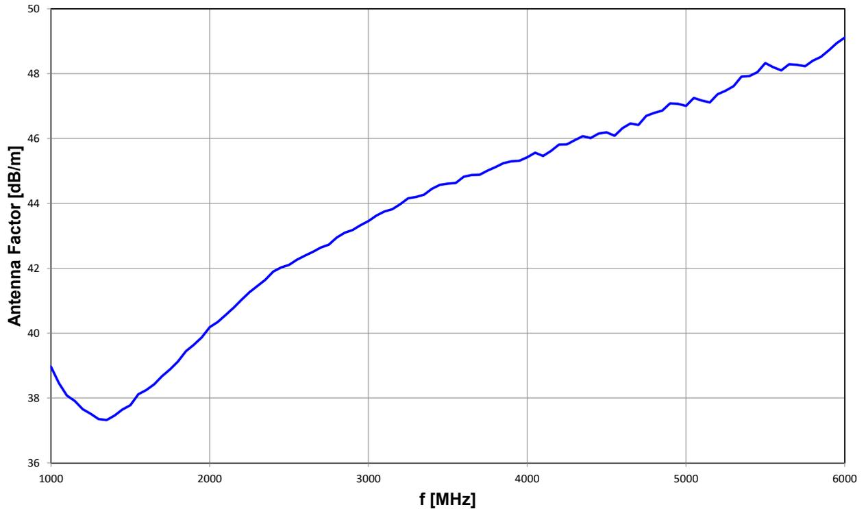
Table 1: Antenna Factor; 1GHz-6GHz, d=3m, Vertical
