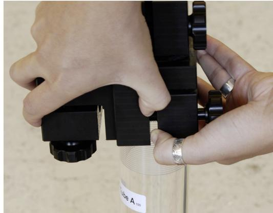
For proper alignment stick the plastic Tube of the POD Holder as far as possible into the HV-Connector front hole. Align the slit of the POD Holder with the mark on the Base Plate and fasten the screw on the HV-Connector to fix it on Tube A.
