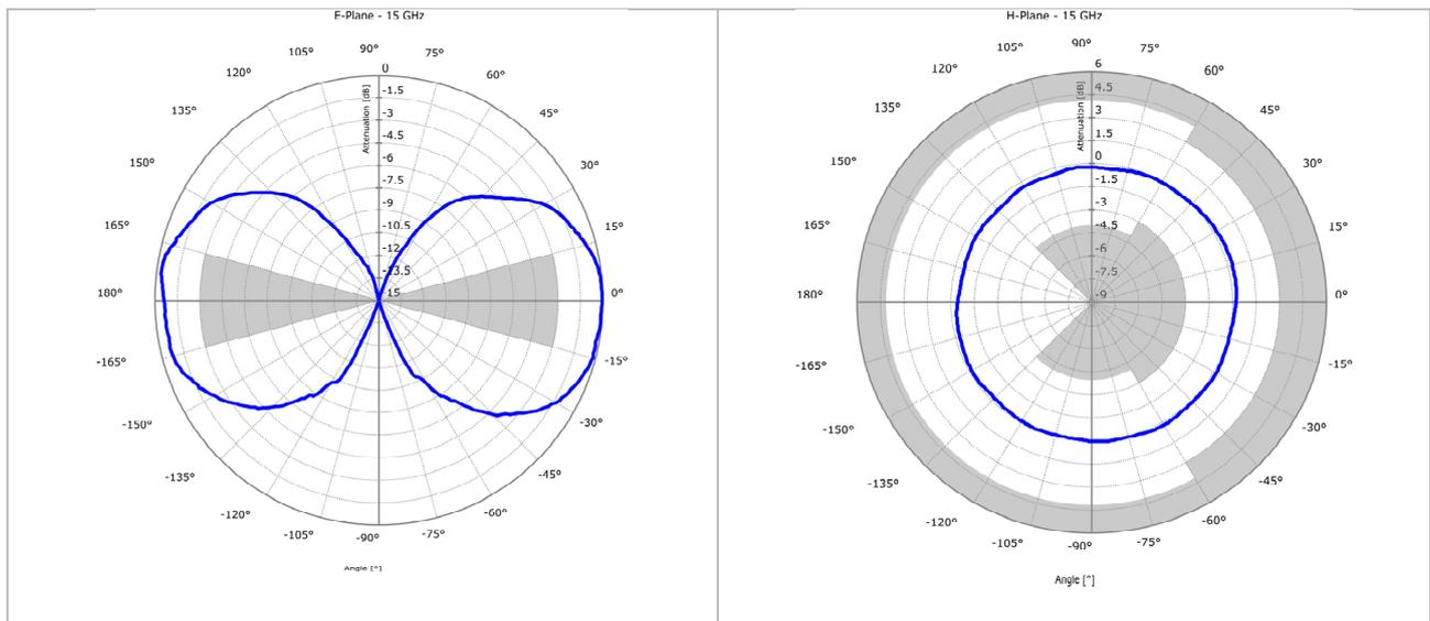
**Figure 3:** Normalized E- and H-plane radiation pattern Results for a POD 618 at 15 GHz and forbidden areas (gray) defined by CISPR 16-1-4.
