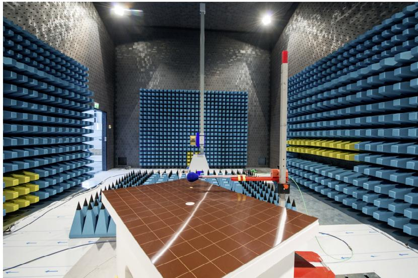
**Figure 20:** Table influence measurement setup 1 GHz – 18 GHz
