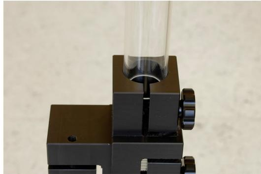
Insert the POD Antenna into the POD Holder. The red 0° marker has to look towards the receive antenna and the white arrow tip has to be aligned with the black part of the POD Holder.
