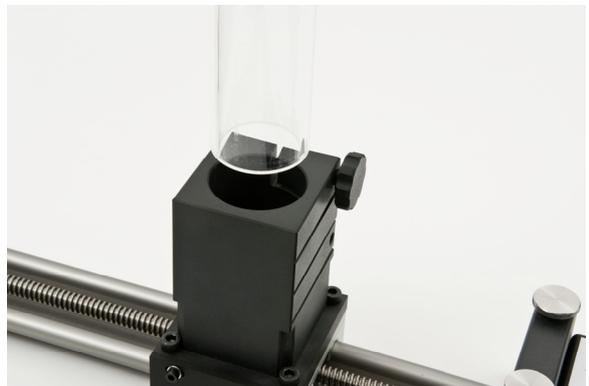
Stick the HV-Connector on the required Tube (you might need to stretch the bracket a bit using your thumbs) – but do NOT fasten the screws.
