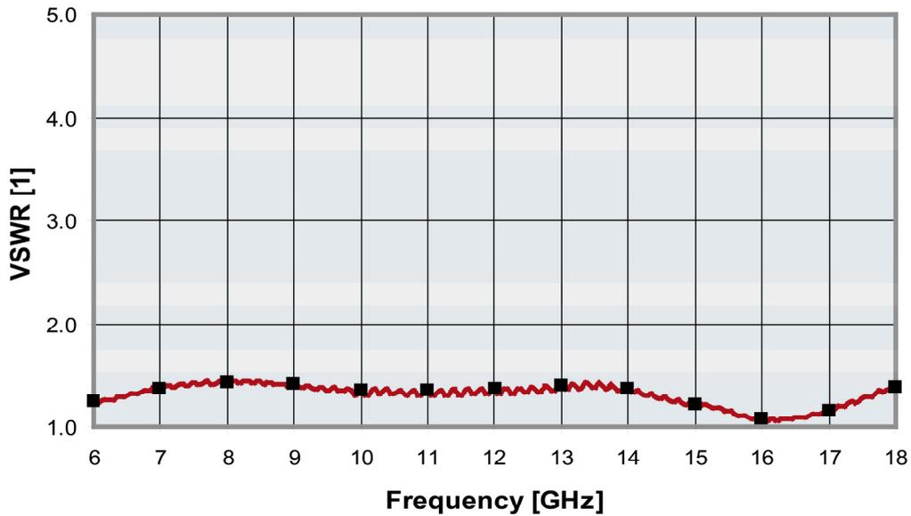
**Figure 14:** Typical Calibration data for POD 618
