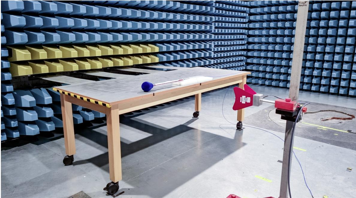
**Figure 23:** ALSE measurement 1 GHz – 18 GHz, horizontal polarisation
