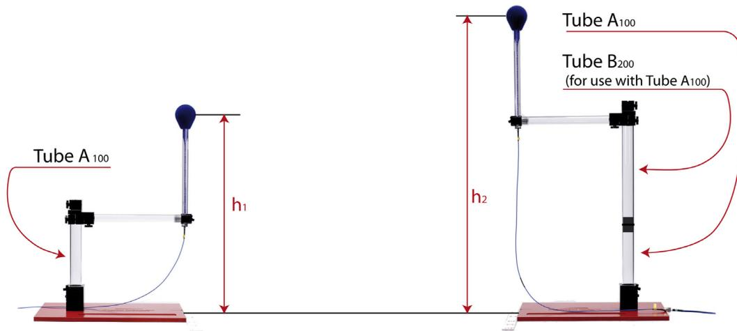
**Figure 18:** Site VSWR Positioner for measuring at  $h_1$  (e.g. 100 cm) and  $h_2$  (e.g. 200 cm)
