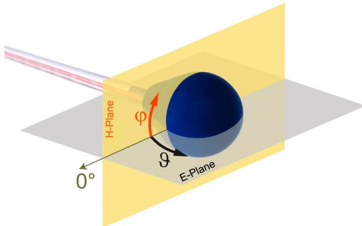
A normalization of the radiation pattern is required by the standard. This is necessary to apply the criteria and is performed for each pattern. For E-plane and H-plane this is done in a different manner:
