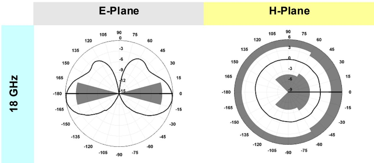
Figure 17: Radiation Pattern POD 618
