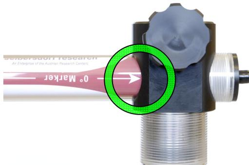
Fix this position with the plastic screw of the POD Holder.
