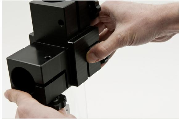
For proper alignment stick the plastic Tube of the POD Holder until it reaches HV-Connector front hole stop. Align the POD Holder to be parallel with the Bracket and fasten the screw on the HV-Connector to fix it on the Tube.
