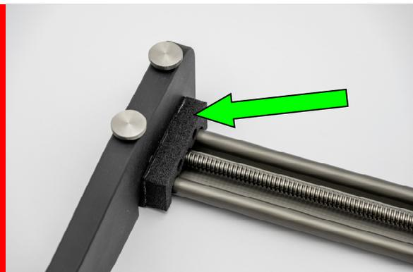
Align the inner edge of the Ruler along the line connecting the 6 test points and adjust the SPA2 so that the marks on the ruler fit to the test points.
