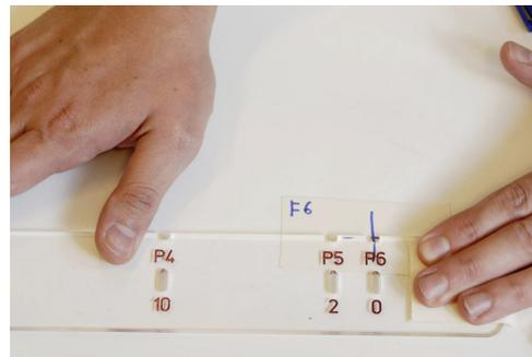
To place the antenna, move the Base Plate along the Ruler until the slot of the Base Plate is aligned with the desired mark on the Ruler.
