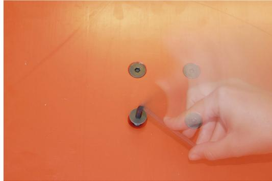
Loosen the 2 black plastic screws on the Tube Base.
