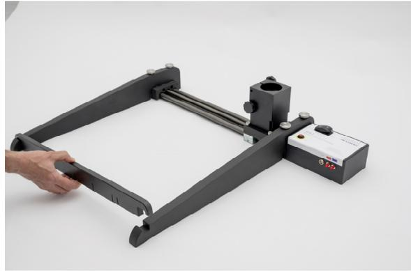
Press the switch "To RX-Antenna >" on the SPA2 box to correspond with the actual position of the receive antenna.
