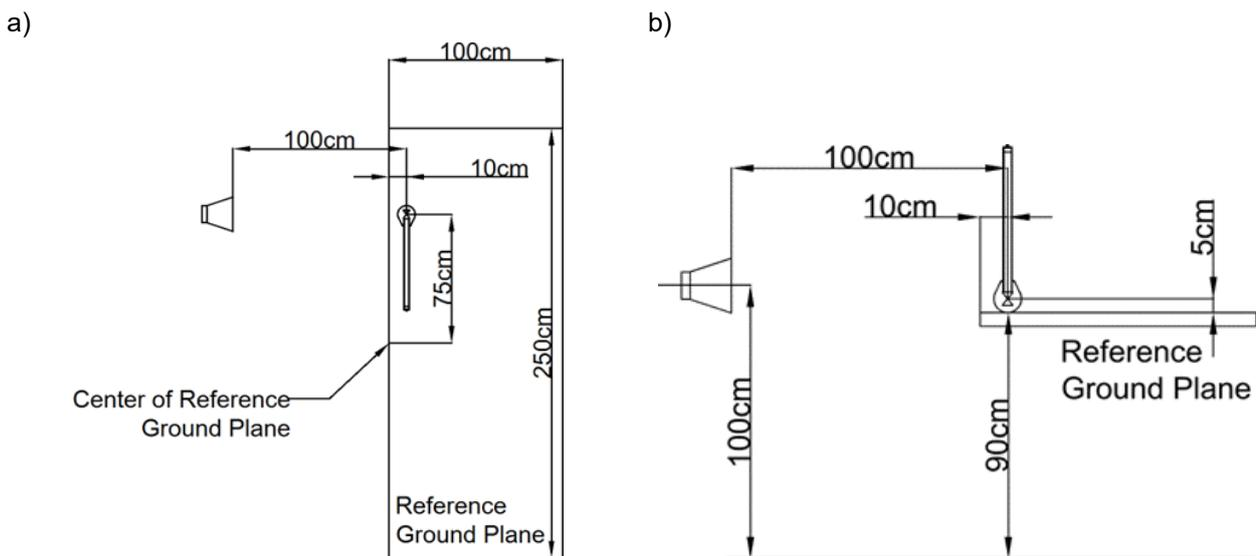
**Figure 22:** ALSE validation setup 1 GHz – 18 GHz
