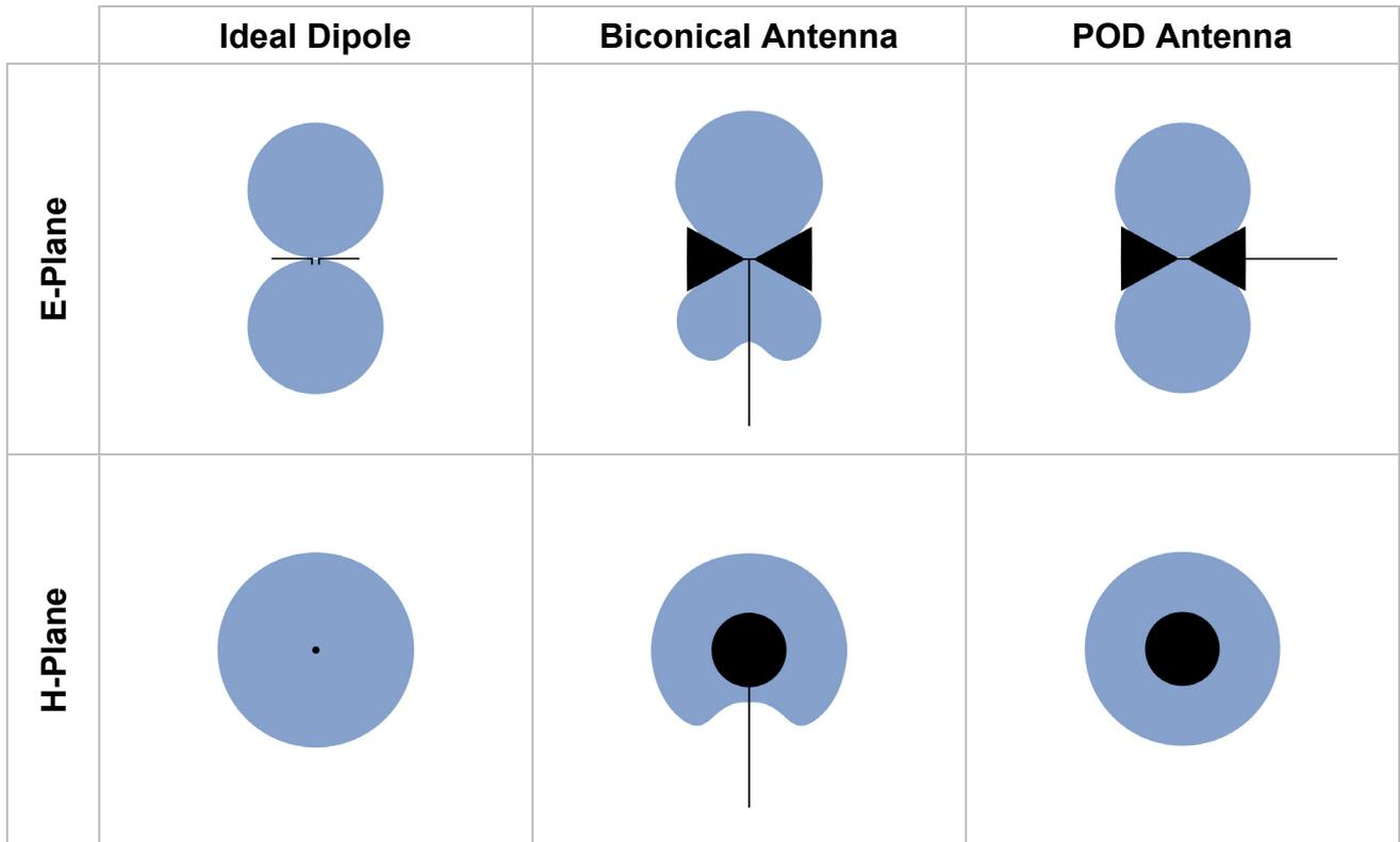
**Figure 2:** Radiation pattern (blue) for different dipole antenna designs (black) in E- and H-Plane. The pattern of the POD Antenna is very similar to the ideal dipole.
