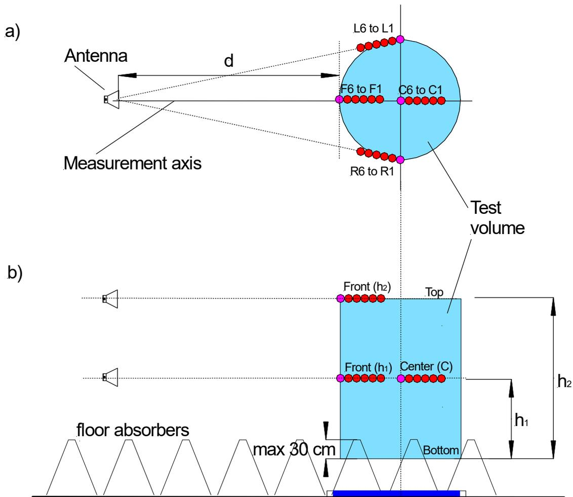
Figure 19: Location of test points for Site VSWR a) top view, b) side view
