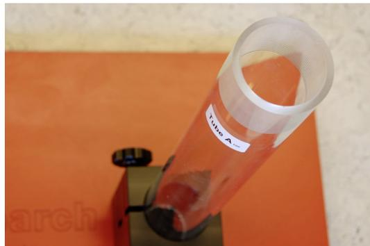
Fasten the two black screws of the Tube Base by hand.
