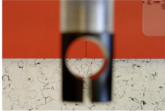
To continue the horizontal setup, remove the POD Holder from the front hole of the HV-Connector and stick it into the top hole.
