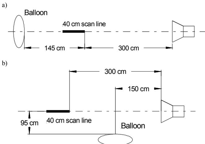
Figure 5. Modified chamber with a) balloon at back b) balloon at side wall
