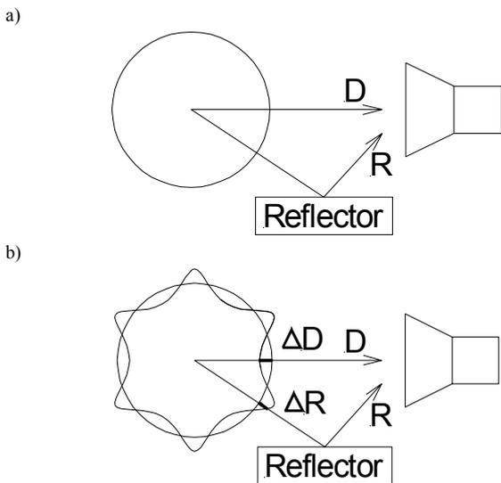
Figure 2. Site VSWR model for a transmit antenna with a a) perfect H-plane pattern b) deformed H-plane pattern
