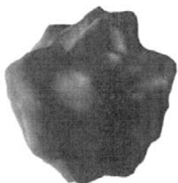
Figure 5: Isotropy of the Add3D procedure using measured radiation patterns of the PCD 8250 antenna
