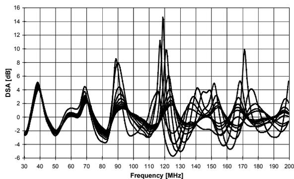
**Fig. 7:** Influence of the limited-size ground plane on the SA dependent on the antenna height. The receive antenna is moved from 1 to 4 m in 30 cm steps
