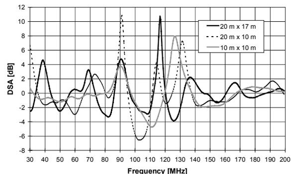
**Fig. 9:** Influence of the ground plane size on the site attenuation.
