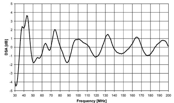
**Fig. 4:** DSA: FDTD simulation for a limited-size ground plane related to a simulated infinite ground plane (NEC).
