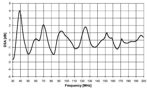
**Fig. 8:** Influence of the limited-size ground plane on the SA when the usual height scan (1-4 m) of the receive antenna is applied to find the maximum received signal.
