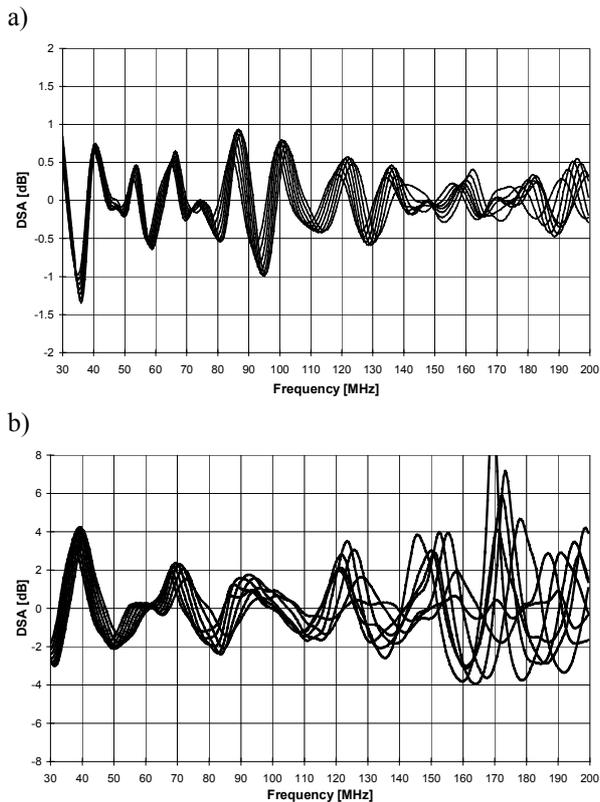
**Fig. 10:** Influence of slight distance variations on the site attenuation: a)  $d=3\text{m} \pm 45$  cm, 15 cm steps; b)  $d=10\text{m} \pm 90$  cm, 30 cm steps
