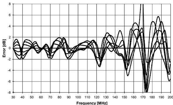
**Fig. 11:** DSA variation when the distance varies in the range 9.1 m to 10.9 m, normalized to 10 m distance on a limited-size ground plane.
