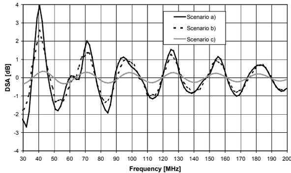
**Fig. 6:** Influence of the limited-size ground plane on the SA. Scenarios as described in Section 3.1.
