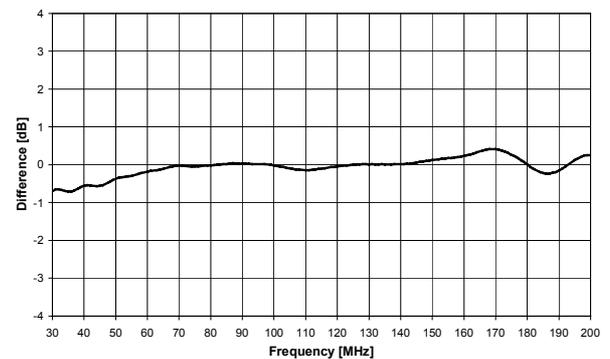
**Fig. 5:** Deviation of the SA results for an infinite ground plane, simulated with FDTD and NEC.
