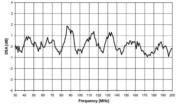
**Fig. 3:** DSA: measurement for a limited-size ground plane related to a simulated infinite ground plane (NEC).
