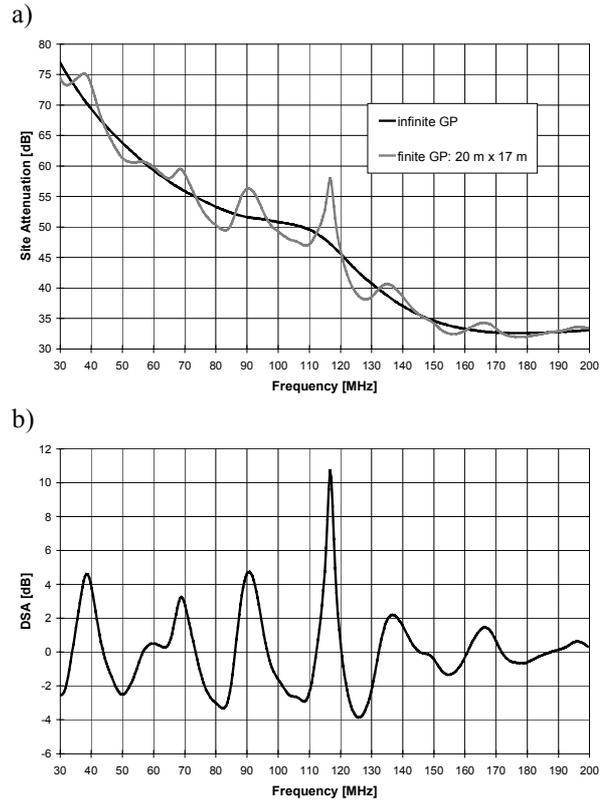
**Fig. 2:** DSA example: a) site attenuation on finite and infinite ground plane; b) deviation of the site attenuation DSA.
