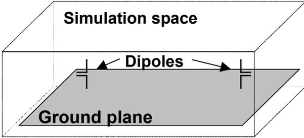
**Fig. 1:** Setup of SA determination on OATS.
