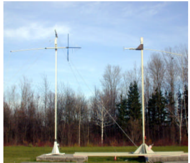
Fig.5 Site Reference measurement on a "Quasi Free Space" site.
