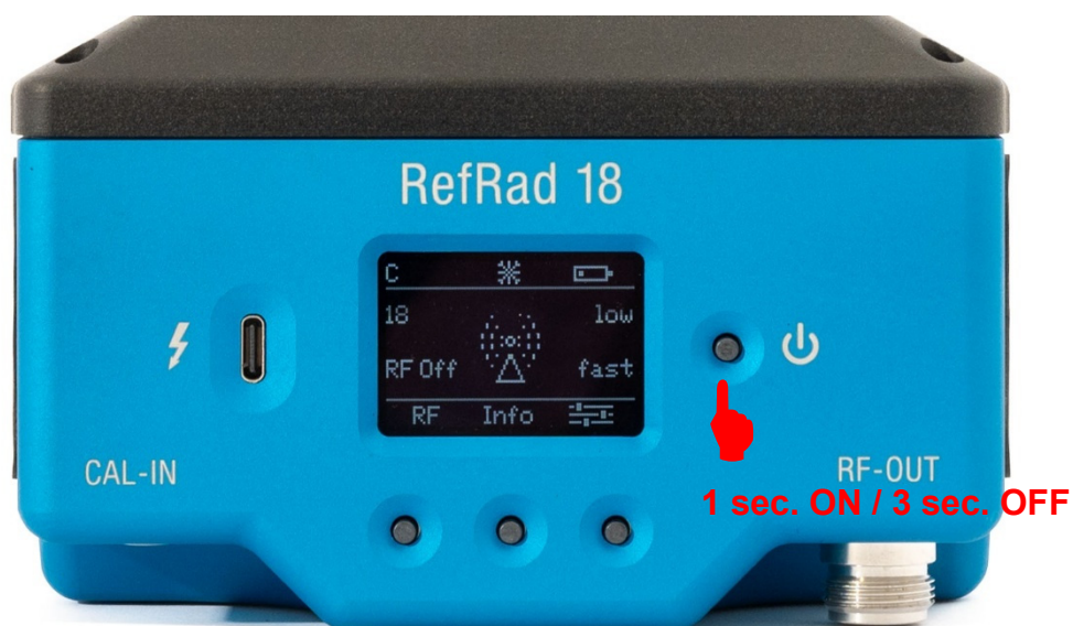
Figure 3: ON/OFF switching process
