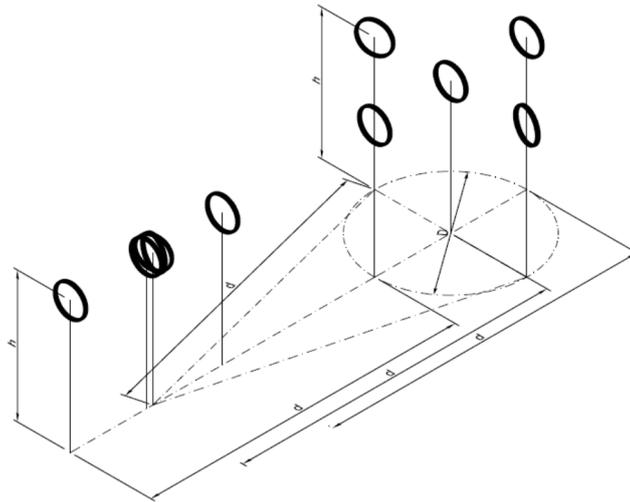
**Figure 26:** Test points inside test volume; orientation  $H_x$  shown
