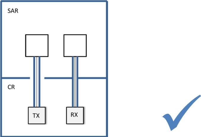
**Figure 29:** Operation of generator and receiver in CR, TX cable not connected to shielding
