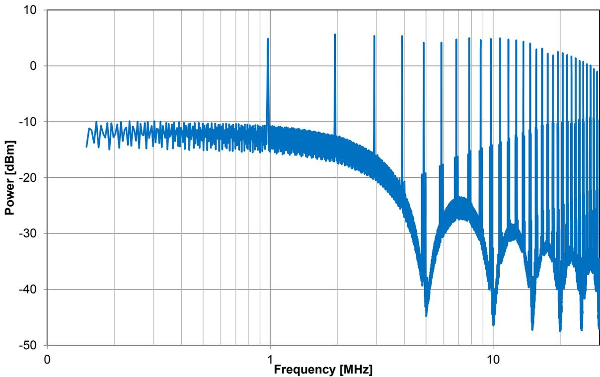
**Figure 16:** Spectrum of pulse generator, CISPR Band B
