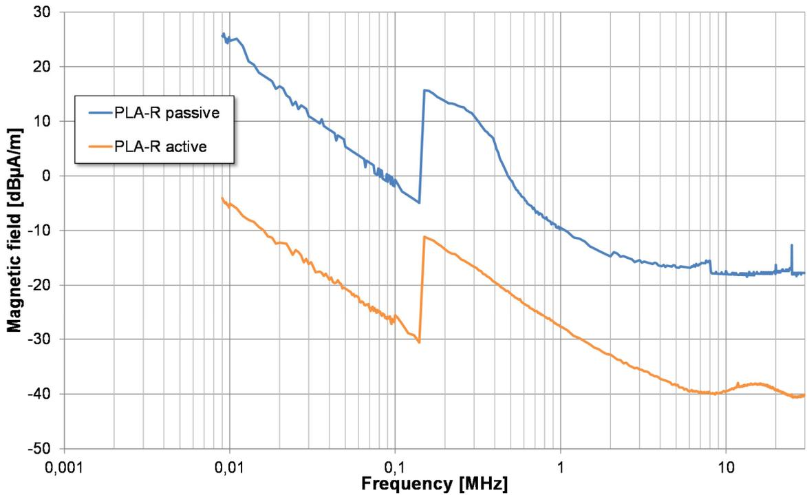
**Figure 13:** Typical noise floor measured with typical EMI Receiver, CISPR bandwidth, Quasi-Peak detector and 10 dB input attenuation
