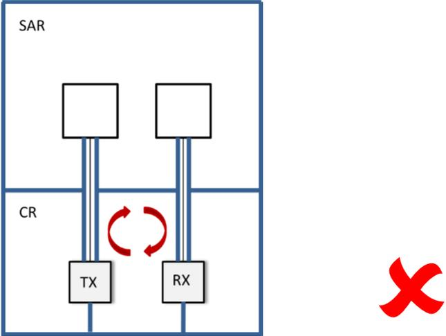
**Figure 27:** Ground loop formed by measurement devices
