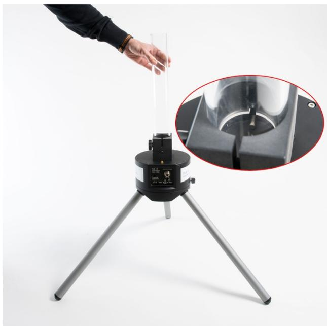
Fix the Tube with the black screw by hand.
