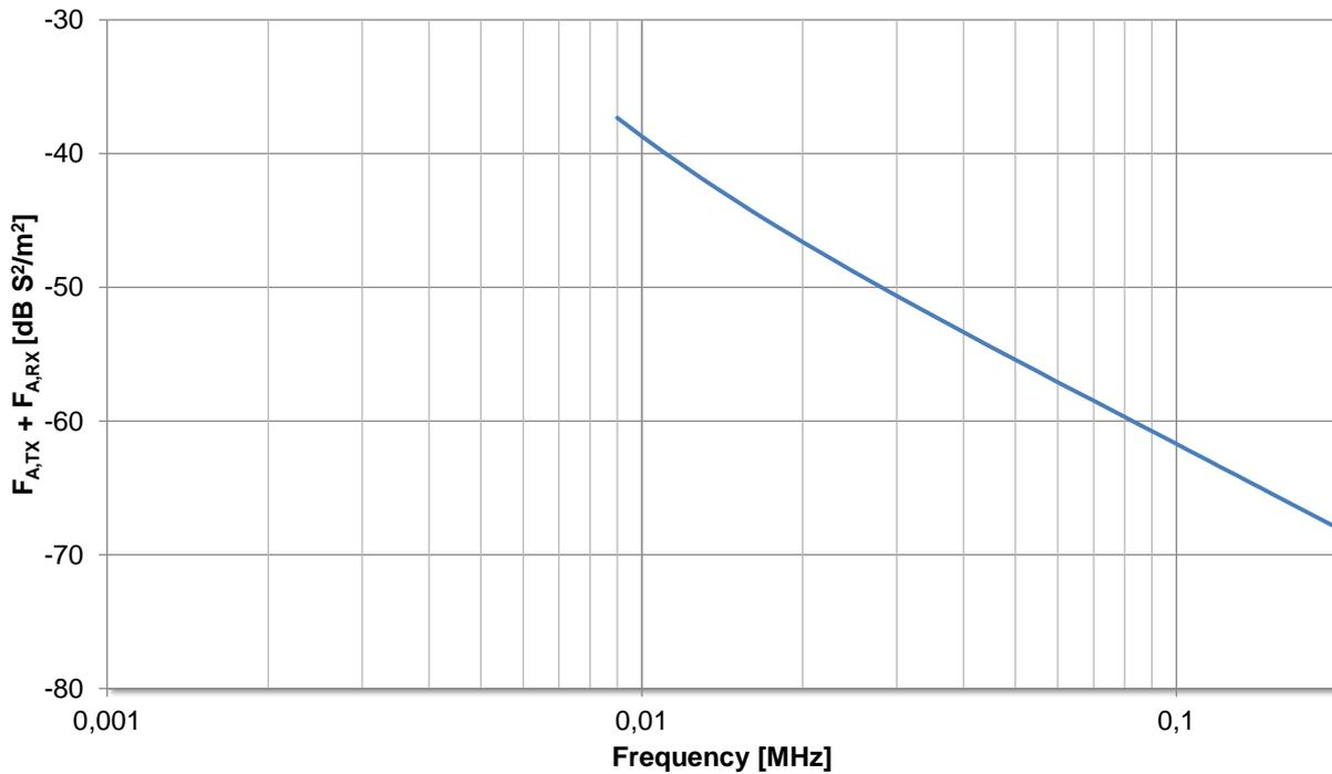
**Table 2:** Sum of Antenna Factors  $F_{a,TX}+F_{a,RX}$  measured at 1 m test distance, TX High current mode, RX Active mode
