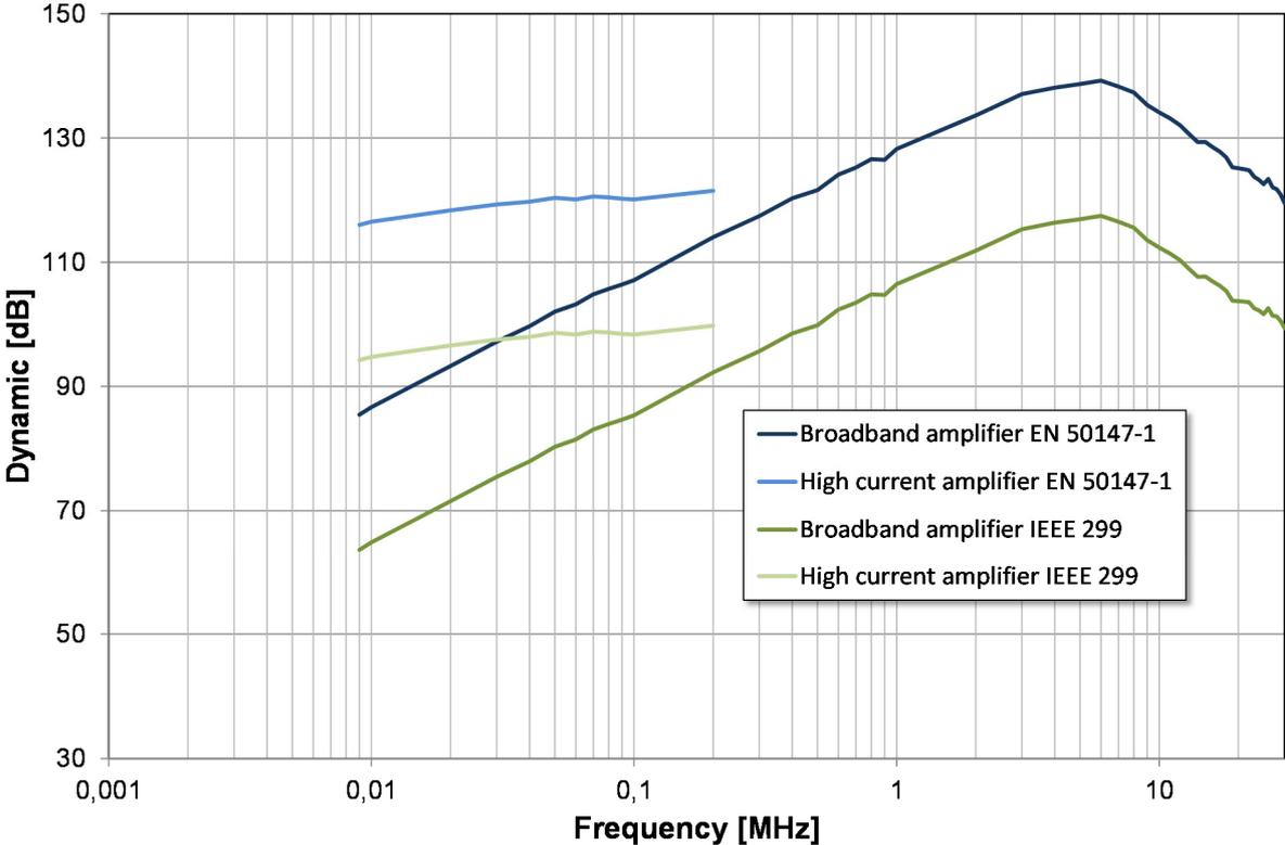
**Figure 34:** Dynamic range; 10 Hz resolution bandwidth
