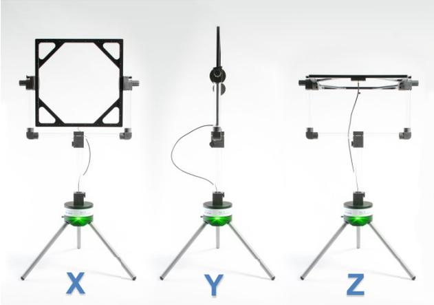
When the antenna is in X-Polarization, turn the Antenna by 90° according to the milling of the Tube to change to Y-Polarisation.
