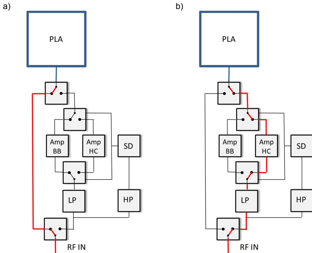
**Figure 6:** Schematic of PLA-T
