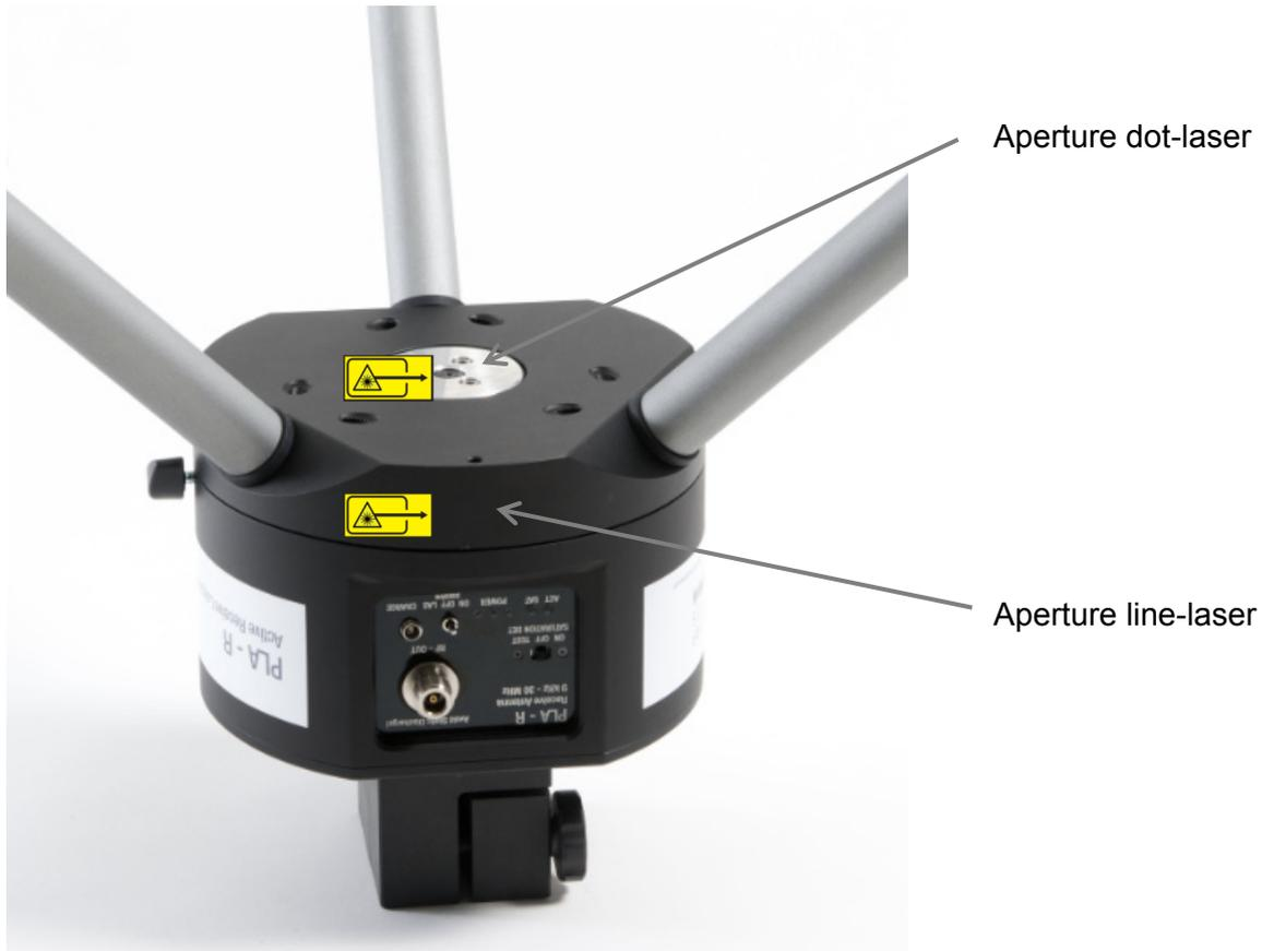
**Figure 35:** Laser Apertures
