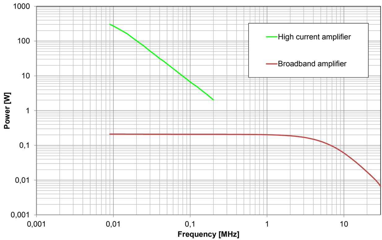
Figure 17: Typical equivalent transmit power in 50 Ω system
