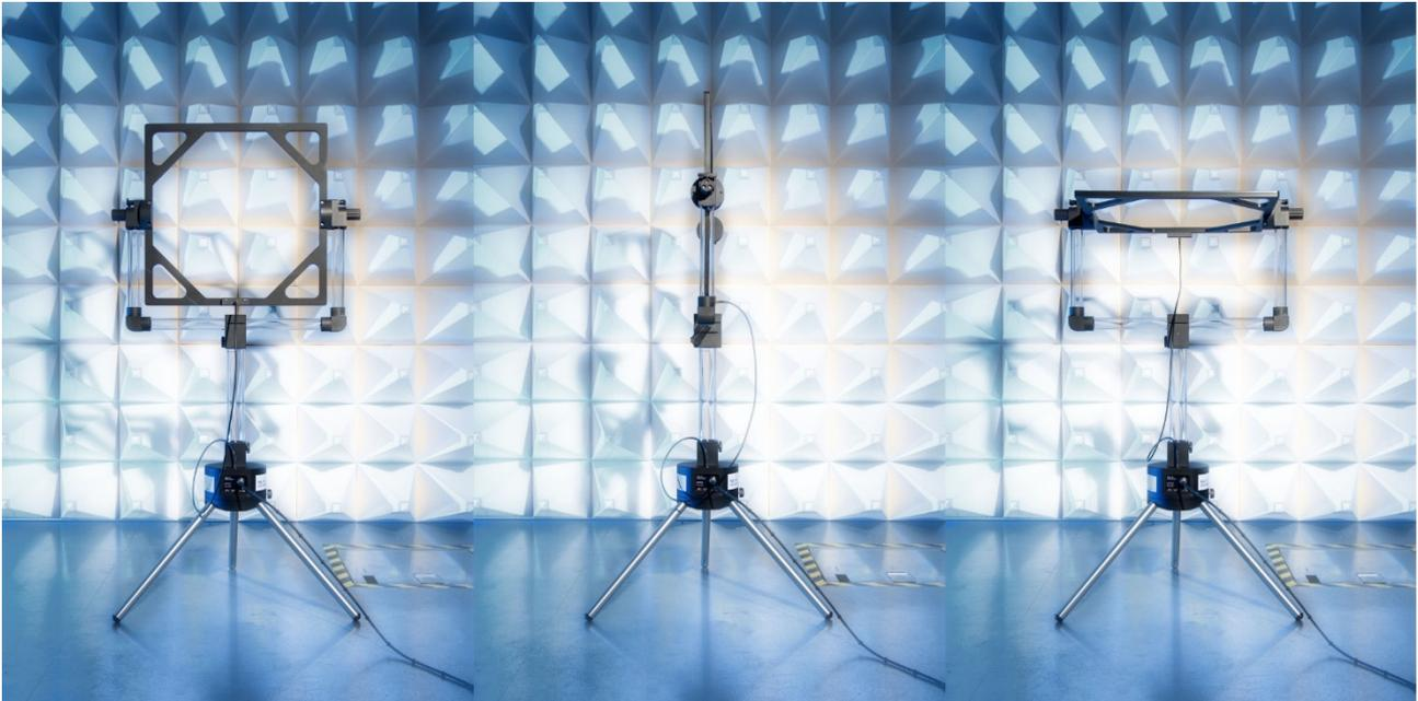
Active **receive** antennas for this frequency range are available since many decades but they all lack of a convenient overload indication which makes them unsuitable for fully automated tests. Design goal was a battery powered active receive antenna that detects overload of the preamplifier on all wave shapes of the RF signals and indicates this on the RF-output in a way that fully automated tests with state of the art EMI-receivers are possible (patented).
