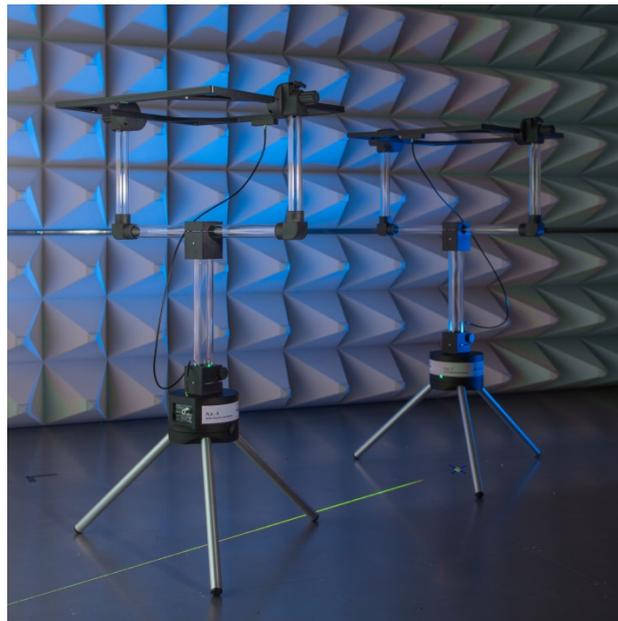
To adjust the line laser release the screw on the Amplifier Box and rotate the case to the target. After the alignment tighten the screw again.
