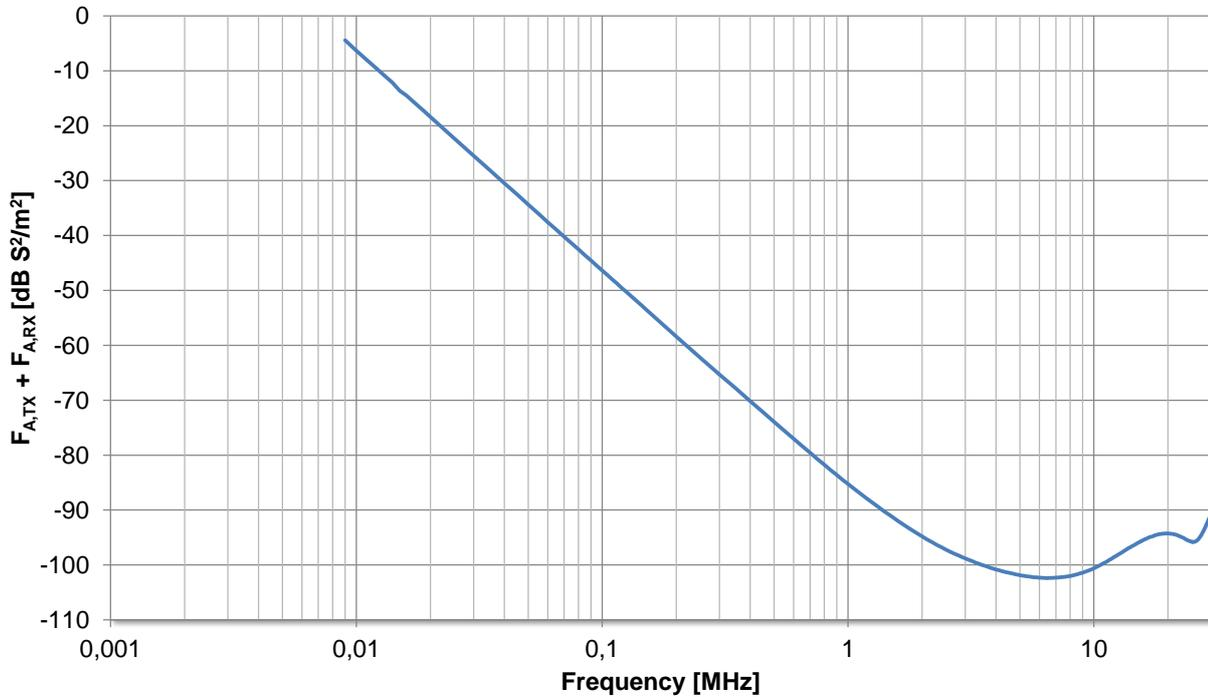
**Table 1:** Sum of Antenna Factors  $F_{a,TX}+F_{a,RX}$  measured at 0.3 m test distance, TX Broadband mode, RX Active mode
