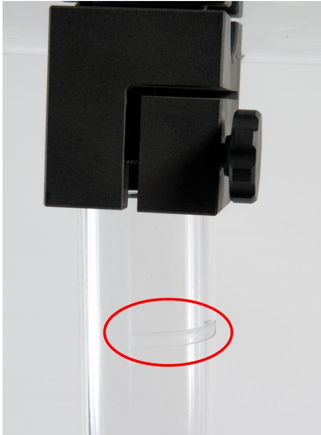
To change to Z- -Polarization, turn the Antenna back to X-Polarisation. Pull out both locking devices and rotate the antenna 90°.
