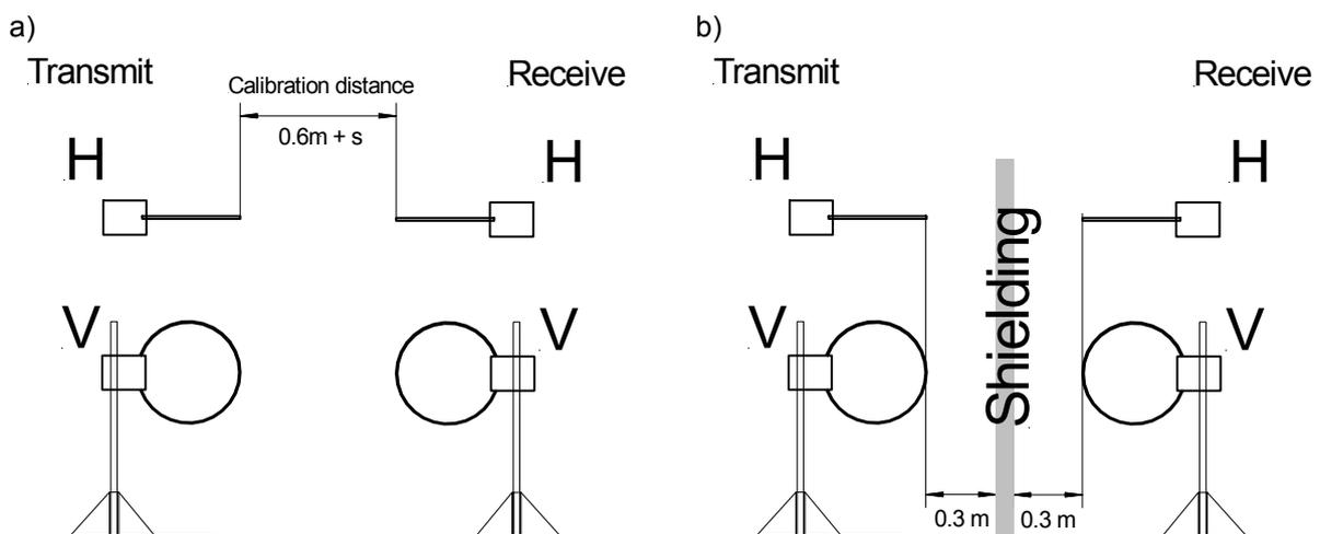
**Figure 33:** Shielding effectiveness measurement setup
