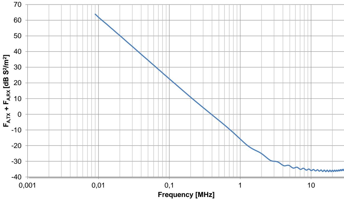
**Table 3:** Sum of Antenna Factors  $F_{a,TX}+F_{a,RX}$  measured at 0.3 m test distance, TX Passive mode, RX Passive mode
