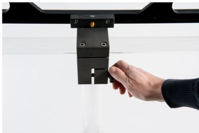
Connect the Antenna cable (SMA connector) to the antenna. Use a torque wrench to tighten the connector-nut.
