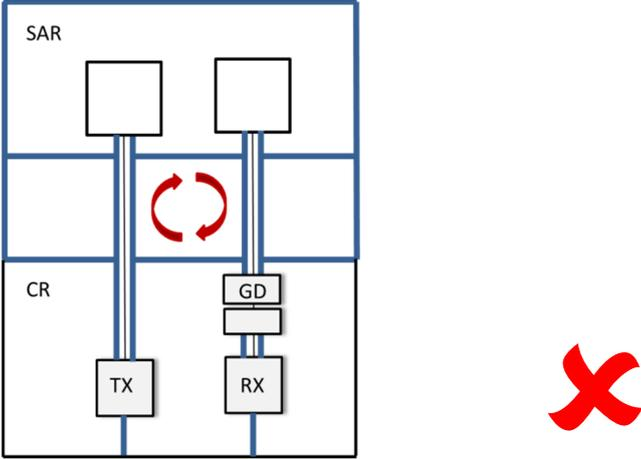
**Figure 32:** Ground loop with fixed installed cables beneath ground plane
