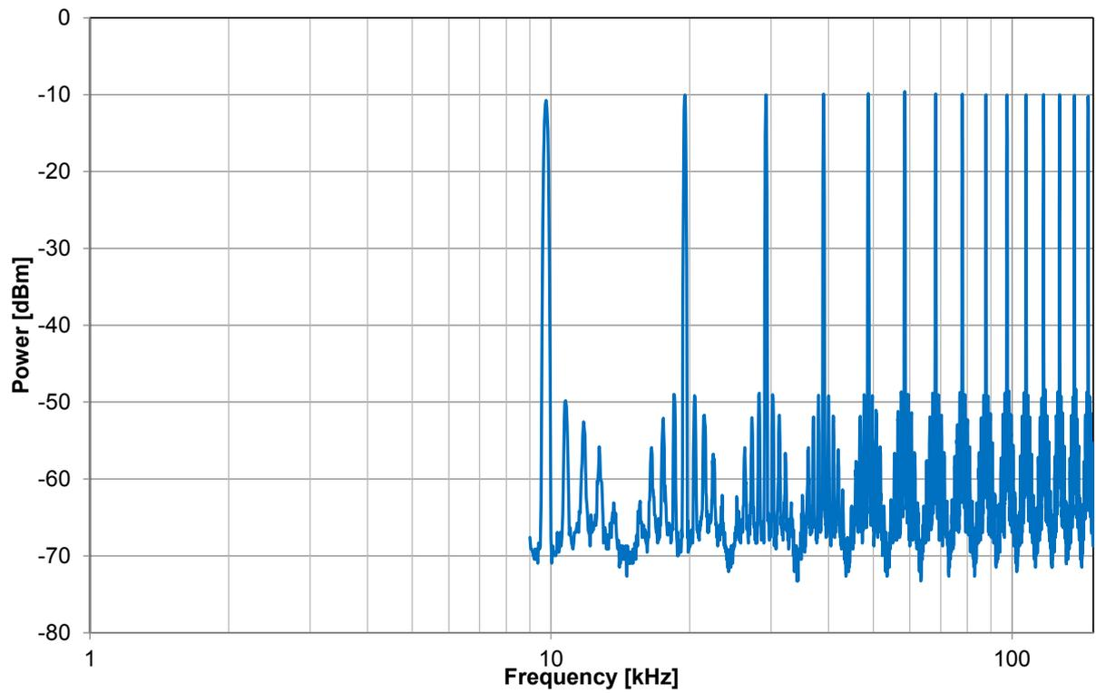
**Figure 15:** Spectrum of pulse generator, CISPR Band A
