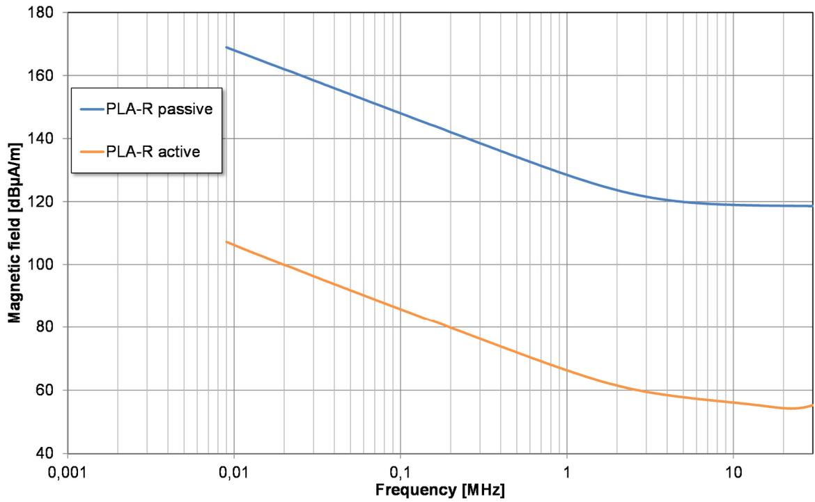
**Figure 14:** Typical maximum field strength; max. +30 dBm on RF input of EMI receiver
