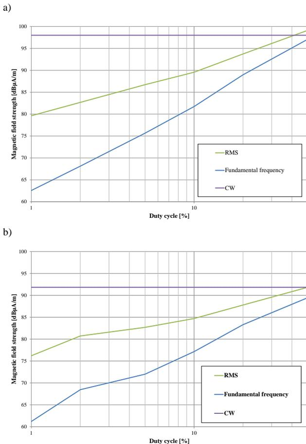
Fig. 7. Measured compression for pulsed signals of antenna a) #1 b) #2
