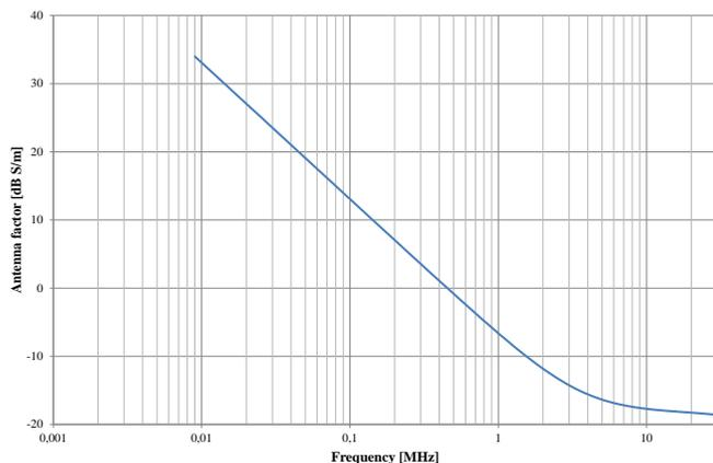
Fig. 9. Antenna factor of a passive loop antenna with 60 cm diameter
