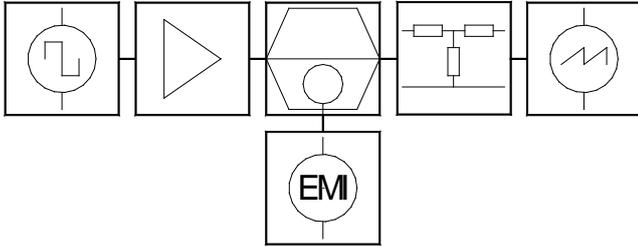
Fig. 6. Block diagram of antenna calibration test setup
