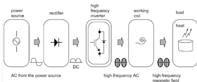
Fig. 1. System topology of EUT from [5]
