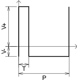
Fig. 2. Shape of a pulsed signal
