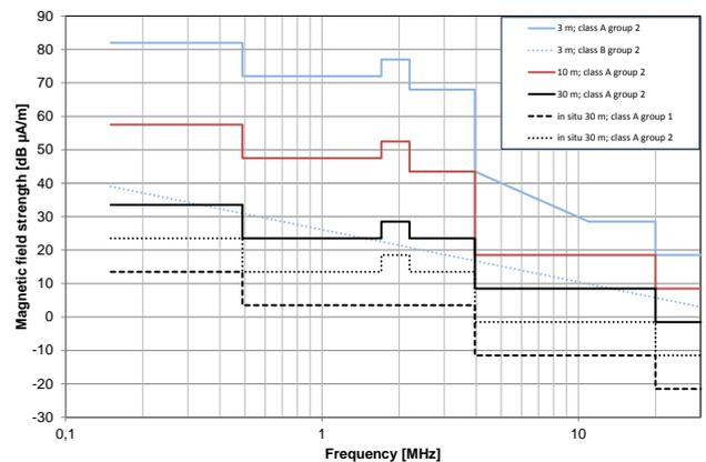
Fig. 5. CISPR 11 emission limits
