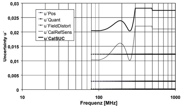
Fig. 5: Uncertainties in the routine sensor calibration by substitution with the reference sensor
