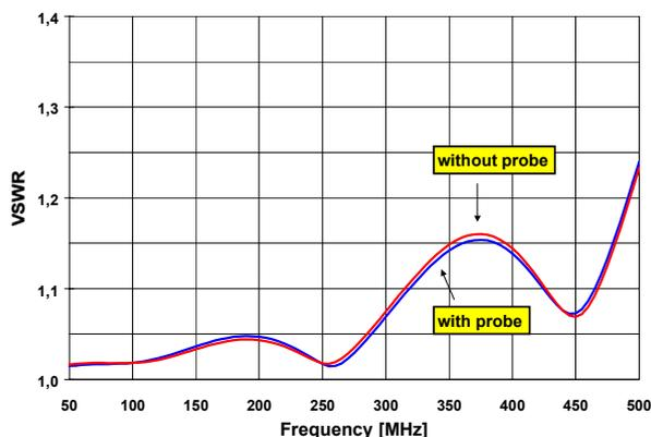
Fig. 1: Standing wave ratio measured at the input of the TEM3 cell of the Seibersdorf Calibration Laboratory
