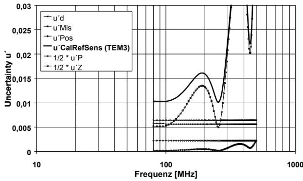
Fig. 2: Uncertainties in the calibration of the reference sensor in the TEM-cell
