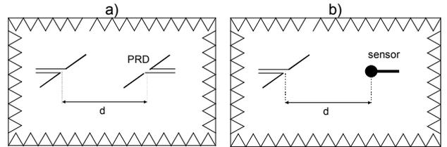
Fig. 3: Calibration of a field sensor in the anechoic chamber by substitution with precision reference dipoles
