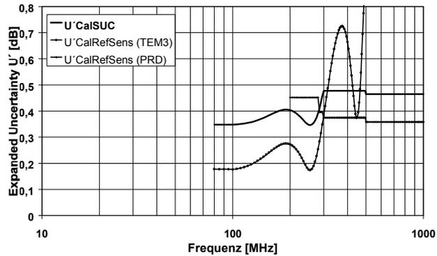
Fig. 6: Expanded uncertainties in the calibration of field sensors
