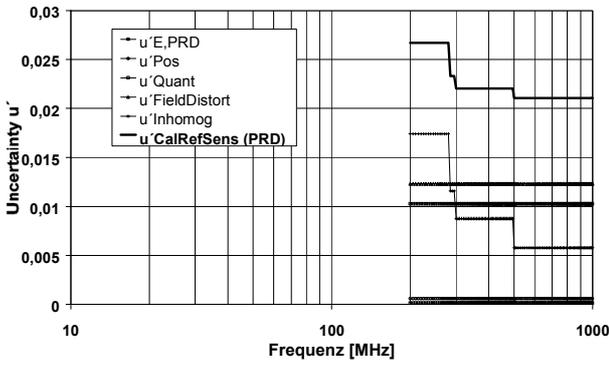
Fig. 4: Uncertainties in the calibration of the reference sensor by substitution with the precision reference dipole
