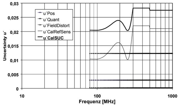
Fig. 5: Uncertainties in the routine sensor calibration by substitution with the reference sensor
